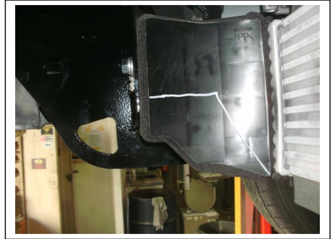
Figure 4: Intercooler air dam trim for under body guard fitment. Right hand side.
