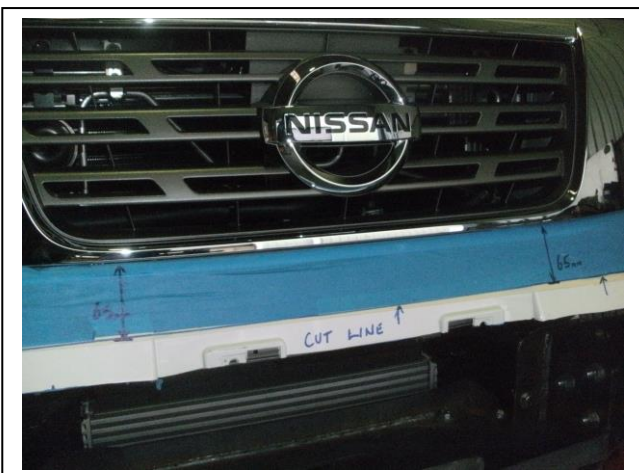
Figure 7: Mark 65mm down from grille as shown
