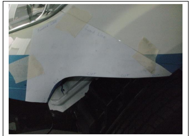
Figure 6: Trim Template in place.
